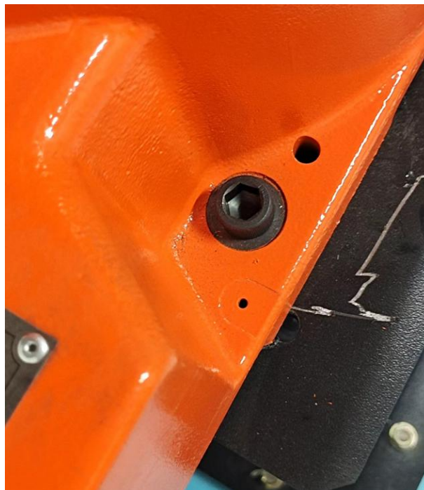
Figure 8.1 Robot base ground connection
