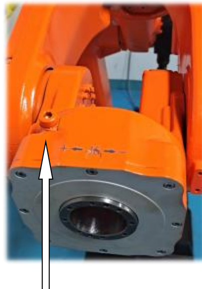
J6 grease drain hole
