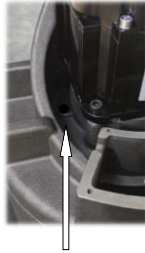
J1 grease drain hole
