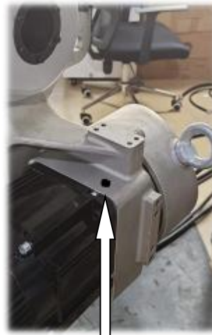
J3 grease drain hole
