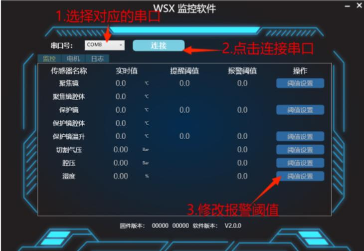
**7.2 Modifying Thresholds:** Click the “ Threshold Settings ” button next to the corresponding sensor. Enter the password “ 666666 ” to access the modification window. The warning threshold must be higher than the alarm threshold.
