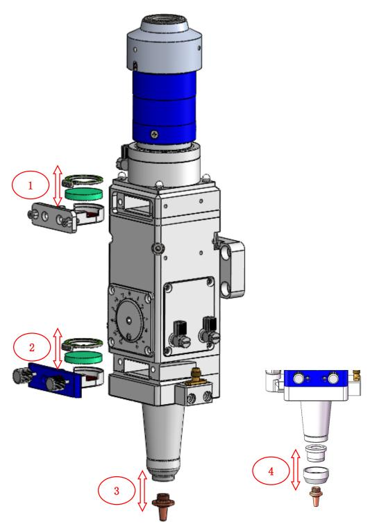
1. Replace the upper dust protection lens: Use a 2.5mm Allen key to loosen the countersunk screws on both sides, and pull out the protective lens cavity seat. Seal the opening of the laser head with a non-adhesive film in time, take out the gland and the waste lens, replace the wiped new protective lens in a dust-free environment, put it in the gland, and replace the protective lens cavity seat.
